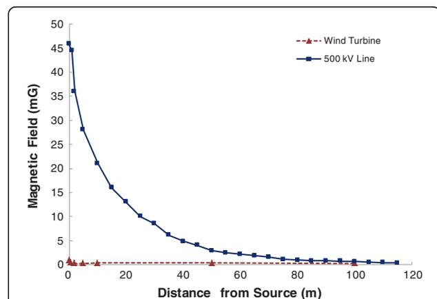
**Figure 3** Comparing magnetic fields around wind turbines and a 500 kV transmission line. Mean magnetic field values have been provided (n = 11) in milligauss (mG). The 'high wind' turbine scenario is presented where conditions were sufficient for power generation.
