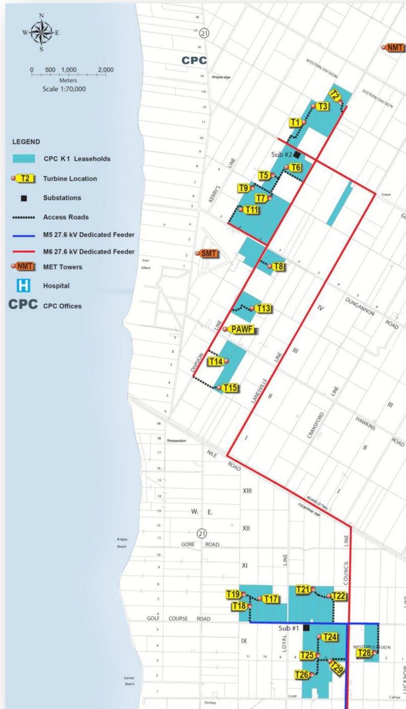
**Figure 1 Map of the study area.** The Kingsbridge (K1) Wind Farm near Goderich, Ontario, Canada. Included are the two substations, collector lines and turbine locations (samples collected around T1-T3, T6, T7, T11, T17, T18, T22, T25 and T29). Samples were also collected around T19, which was non-operational (not connected to the grid) and was used in this study as a control.
