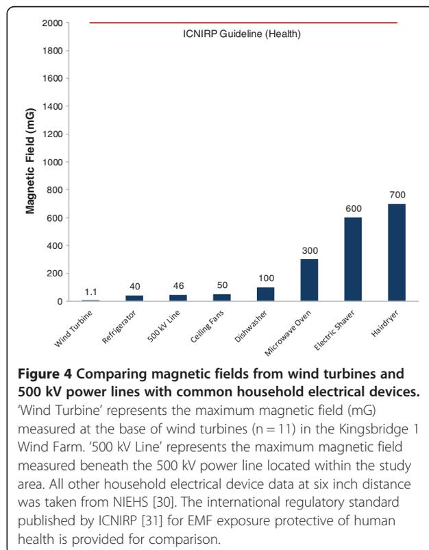
**Figure 4 Comparing magnetic fields from wind turbines and 500 kV power lines with common household electrical devices.**
