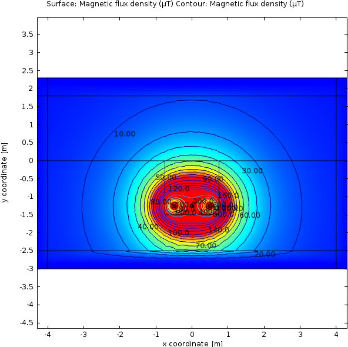
Fig. 3. Magnetic flux distribution around the cables; Y coordinate=0 symbolizes ground level.
