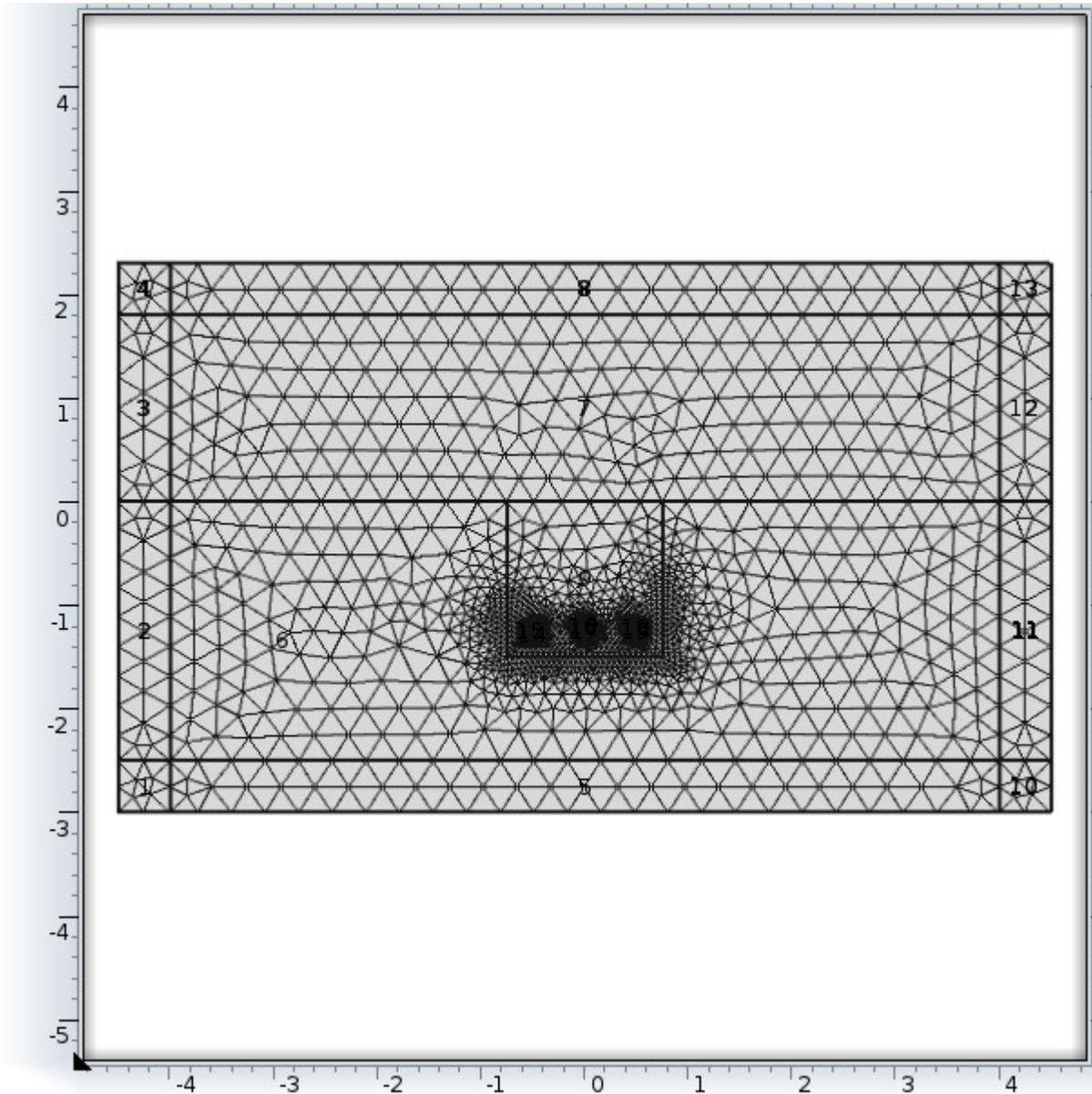
Fig. 2. Mesh and contours of the cable installation model; the coordinates are expressed in meters [m] (see next figures)
