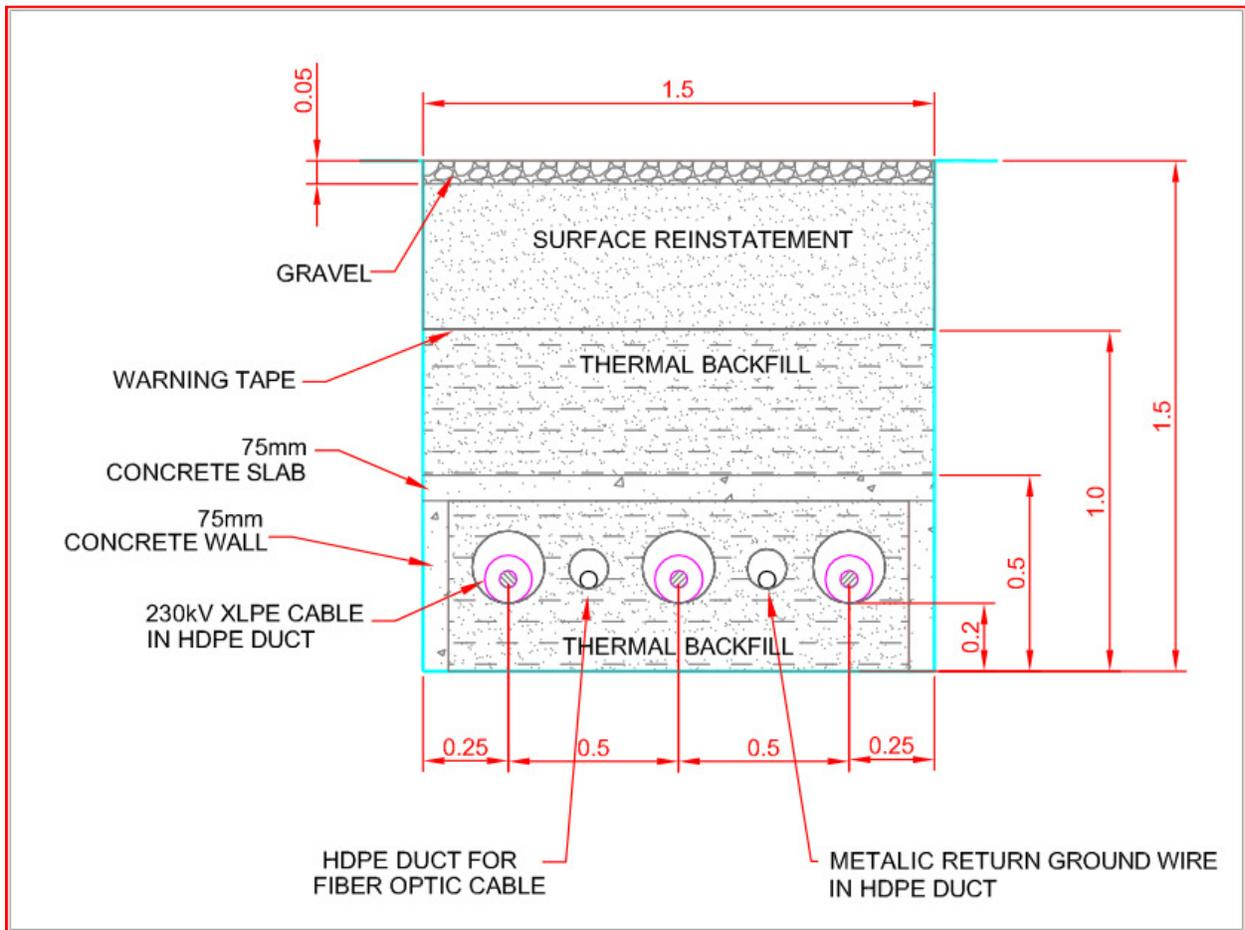
Fig. 1. Cable installation provided by Genivar
