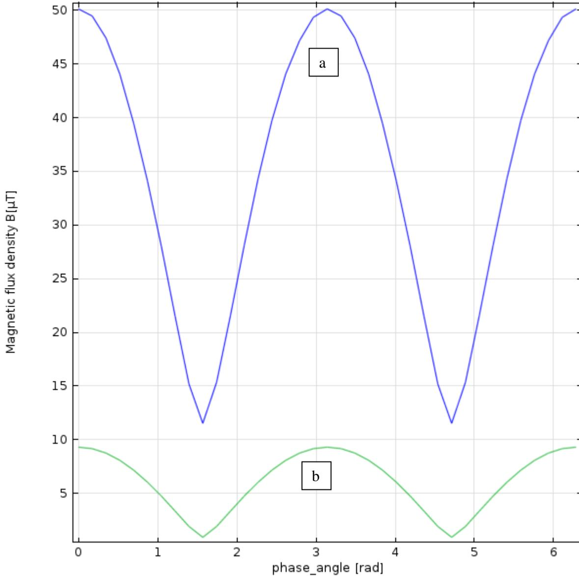
Fig. 4. *Magnetic flux density as a function of the phase angle (which determines an instantaneous value of the current)*
